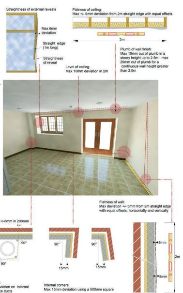
Figure 6: Maximum deviation in walls and ceilings
